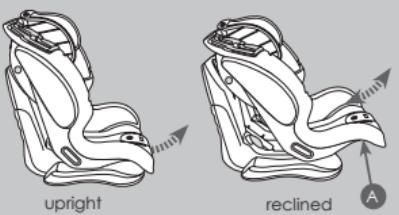
The child car seat can be used in four different seat positions, from seated to a reclined sleeping position. Pull the recline adjuster handle (A) under the front of the shell and pull the shell forwards or backwards, release the handle on your required position when hearing a distinct click.
