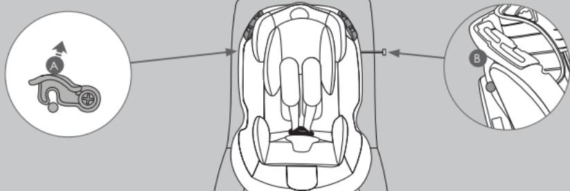
Release catch (A) on the top left hand side of the shell and remove the installation bar (B).
