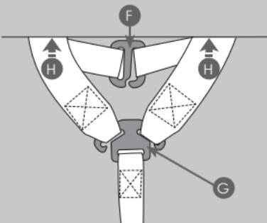
Unhook the shoulder pad straps from shoulder pad connector (F).
