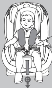
After placing your child in the child car seat, match the two halves of the harness buckles together and insert them into the crotch buckle.
