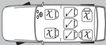
The child car seat can only be used with an automatic 3-point safety belt (A) and **NOT** with a 2-point lap belt (B).
