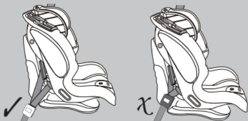
With your child car seat now buckled in, check it is secure by pulling forward from both harness straps, there should be little or no movement. Next check that the vehicle's seatbelt buckle is NOT resting against the child car seat shell. This is called 'buckle crunch' and could cause the child car seat to work loose or the seatbelt to come
