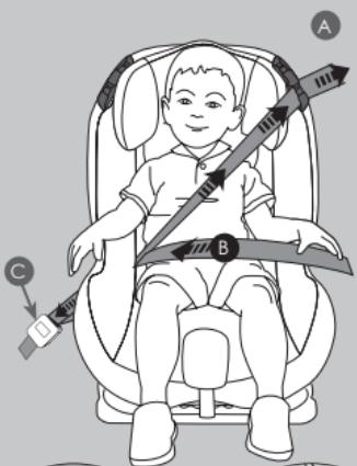
Place the seatbelt shoulder strap through the most suitable belt guide slot (A): Use the lower strap hook for children in group 1 (15 - 25kg).
