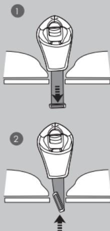
To remove the crotch strap, ensure the child car seat is in a fully reclined position.
