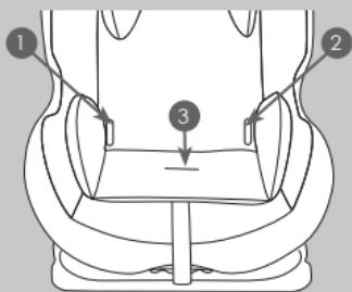
Insert waist strap retainer buckles (C) through the two slots (1) and (2) on the cover and out through the outer slots on the back of the shell then back through the inner slots.
