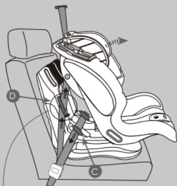
Push the child car seat back into the passenger seat ensuring a good fit. Thread the horizontal lap belt section under both hooks (C) and remove all the slack by pulling up on the diagonal section of seatbelt. Thread the diagonal section through the lock off device (D) that is nearest to the seatbelt.
