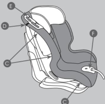
The main cover is held in place by a series of hooks (C) located on the back and underside of the shell. Unhook the cover's elastic from the hooks. Undo the Velcro® tabs (D) on the shoulders of the shell, work the cover from under the strap hooks (E) and from around the plastic adjuster panel (F) and remove the cover.
