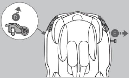
Release catch (D) on the top left hand side of the shell and remove the installation bar (E).
