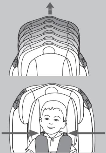
Adjust the headrest by pulling the adjuster handle on the back of the headrest and raising or lowering according to your child's height.
