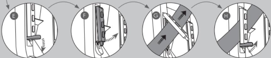
To operate the lock-off device: Pull down on tab (E) to open the locking device. Lift up the latch (F). Pass the seatbelt under the latch and pull the belt tight (G). Close the latch and fasten the tab (H) whilst holding the diagonal section of seatbelt tight.
