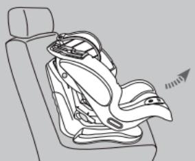
Place the child car seat on a suitable passenger seat. Pull the recline adjuster handle under the front of the shell and adjust the shell to its fully reclined position.
