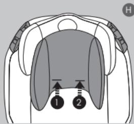
**ATTENTION:** The shoulder pad and harness straps **MUST** pass over the metal bar, failure to do so will result in an incorrect installation.
