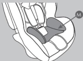
Remove the booster cushion insert (M) from the crotch strap.
