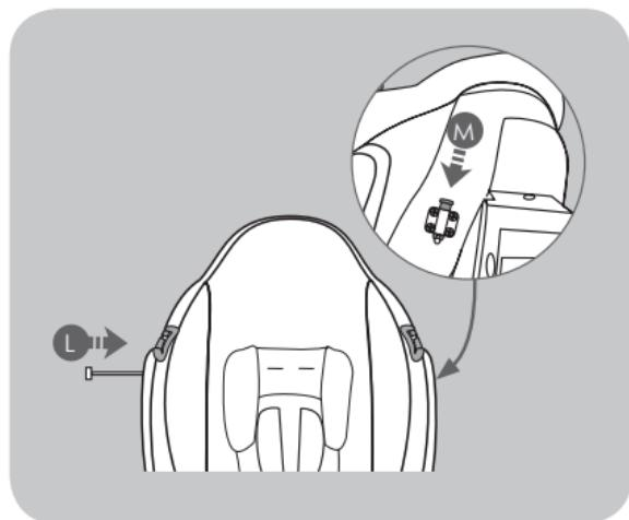
Return the shell to its original position and re-insert the installation bar (L) and secure lock (M).
